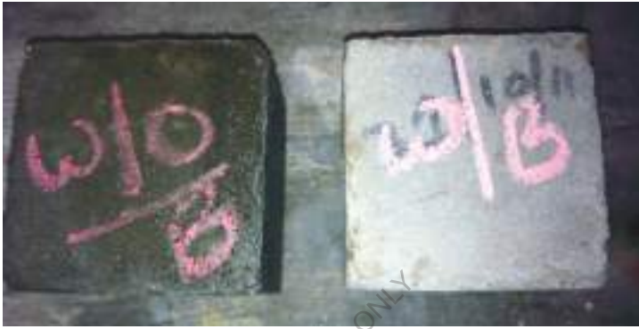
Figure 8.2 - untreated and bacteria treated surfaces of mortar cubes
