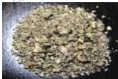
Fig 2 - GBFS Sand (Source: JSW slag, Bellary)
